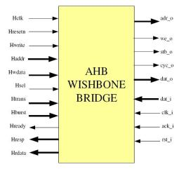
*Figure 1: The AHB-2-Wishbone bridge – an OpenCores design*
