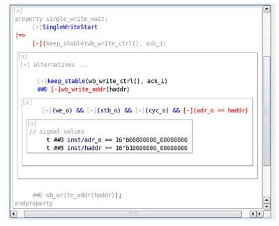
*Figure 4: The StructuralAssertionAnalyzer automatically identifies failing parts of the assertion (Source: OneSpin)*
